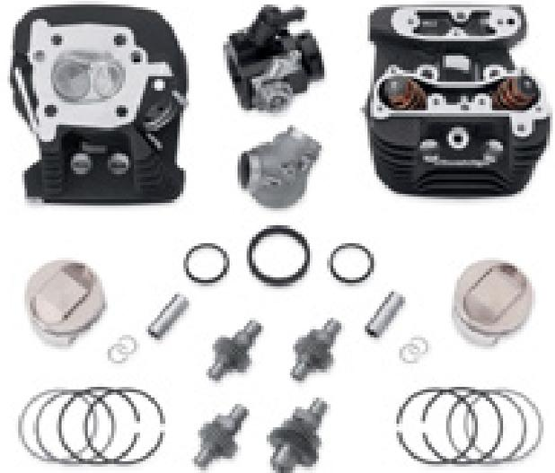
Stage IV "bolt-on" upgrade requires removal of the engine's top end and opening the cam chest. Engine remains in the chassis and no machining is required. Special tools and ECM tuning are required.
