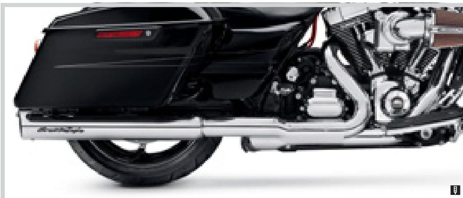
**B. SCREAMIN' EAGLE HIGH-FLOW EXHAUST SYSTEM WITH STREET CANNON MUFFLERS – CHROME (SHOWN WITH SHORT SLASH OUT END CAPS)**
