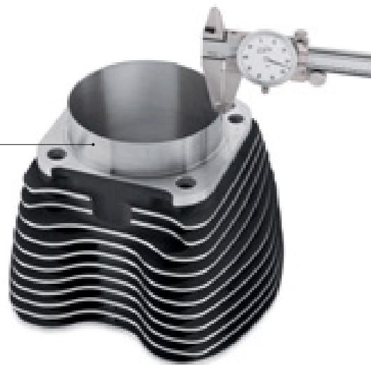
HIGH-STRENGTH CYLINDER LINERS ARE MACHINED TO SLIP INTO THE STOCK CASE OPENING
